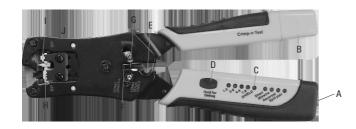
A. UTP/STP Cable Test Jack
